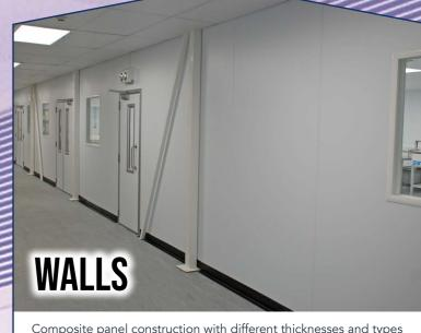
Composite panel construction with different thicknesses and types of insulation, panel faces manufactured from powder-coated steel varying in coating application, dependent on chemical and scratch resistance required. Semi flush and fully flush systems available, wall-to-wall and wall-to-ceiling coving as standard.
