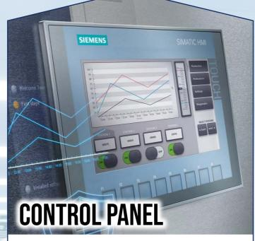
Touchscreen HMI provides the interface for the controls and monitoring systems for your cleanroom. The EMS feeds back to give real-time data on temperature, humidity and pressure. The BMS can link back data concerning the operational status of all plant, including fan speeds, coil condition, run data and other connected utilities.
